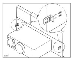
■ When fitting a DA 3190 into a 60 cm housing unit, unscrew the brackets on the deflector plate whilst it is pulled out.
